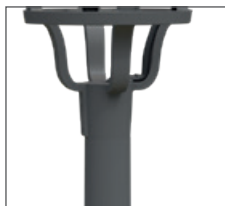
Supported: Pole top fixing Ø 60 mm Len 70 mm, 2 self-centring screws
