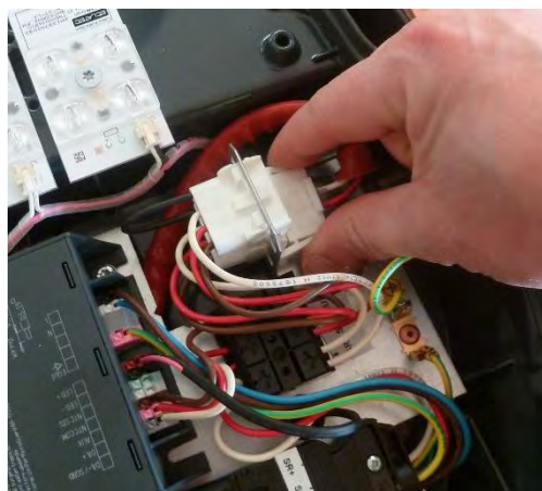
F - Disconnect the superior Zhaga wiring harness of the gear tray.
