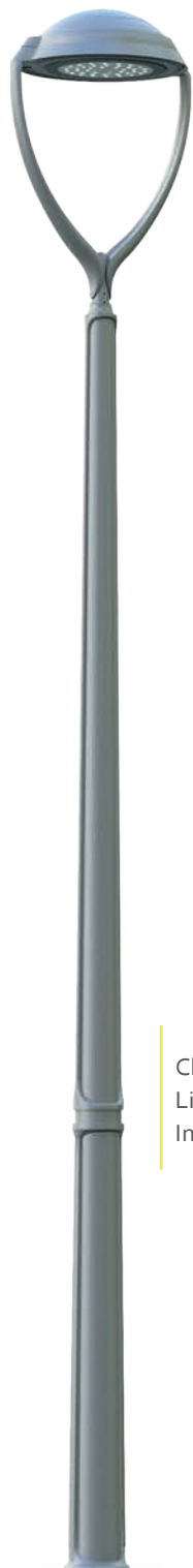
Arcos GI 13 pole Lighting height 7 m Overhang 1.50 m
